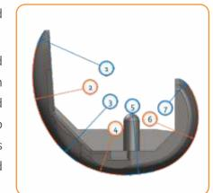
Radii 4, 5, 6 and 7 control femoral rollback and flexion over a wide array of biomechanical requirements, from walking to climbing stairs & ensure optimized area contact for uniform load dissipation both in extension & flexion thereby minimizing the contact stress.
