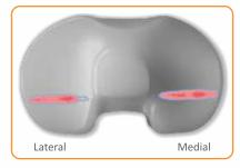
Representative Surface Stress Distribution 15 - 40 + MPa at 90 Degree Flexion, 333 kgf Load
